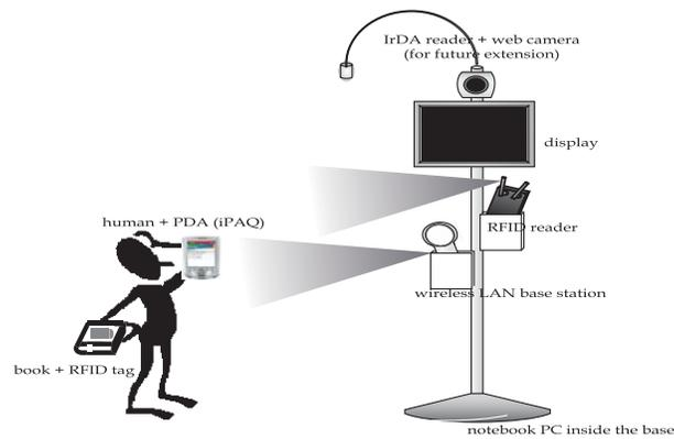
**Fig. 6.** Hardware Configuration of the Prototype System
