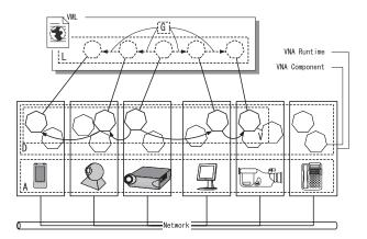
Fig. 5. Virtual Networked Appliance Architecture
