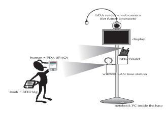
Fig. 6. Hardware Configuration of the Prototype System
