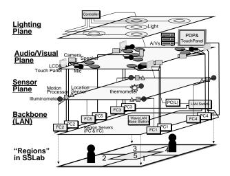
Fig. 3. Embedded Sensors, Appliances, and Networks in B-in-B
